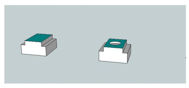
Step 4. Drill hole for the spindle collar 3/16" deep with a 1 1/4" Forstner bit.
