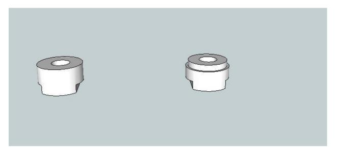
Step 12. Glue the PVC adapter to the hub with epoxy or another suitable glue. After the glue is set, remount and turn the base down to the size of the PVC adapter.
